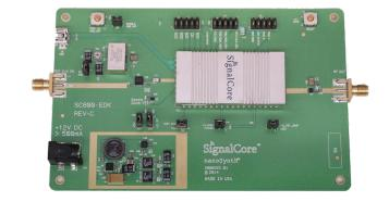
Frequency Range 25 MHz to 6 GHz -112 dBc/Hz at 10 kHz offset, 1 GHz carrier Phase Noise Tuning Resolution 1 Hz (exact frequency) Spurious Signals -65 dBc typical 2nd order harmoncs -15 dBc typical
